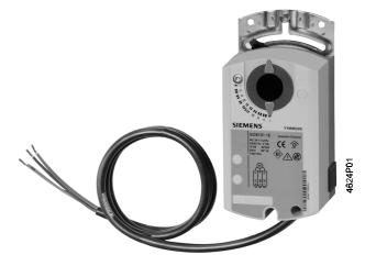
Electric motor-driven actuators for three-position control, 5 / 10 Nm nominal torque, AC 24 V or AC 230 V operating voltage, mechanically adjustable working range between 0...90°, pre-wired with connecting cables of 0.9 m.
